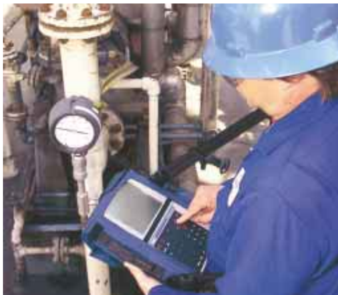
Microlog – portable data collector and analyser
