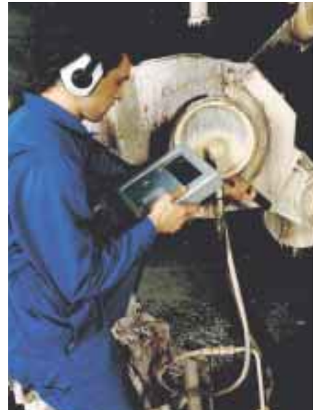
Recording vibration values using an SKF Microlog data collection unit
