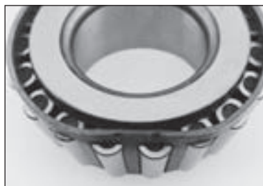
Cage deformation — Improperly installed or dropped bearing.
