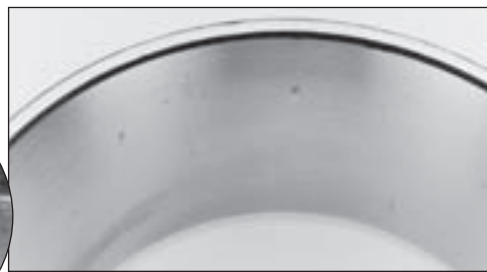
Roller spaced nicking — Raised metal on races from contact with roller edges.
