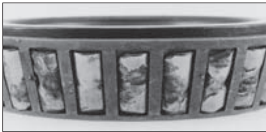
Rapid and deep spalling caused by unusually high stresses. Full race width fatigue spalling is caused by heavy loads creating a thin lubricant film and possible elevated temperatures.
