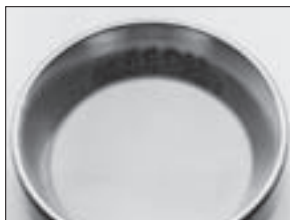
Irregular roller path from deflection, inaccurate machining or wear of bearing seats.
