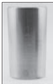
Roller nicking/denting — Rough handling or installation damage.
