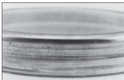
Cup spinning — Loose cup fit in a rotating wheel hub.
