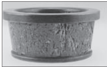
Rapid and deep spalling caused by unusually high stresses. Full race width fatigue spalling is caused by heavy loads creating a thin lubricant film and possible elevated temperatures.
