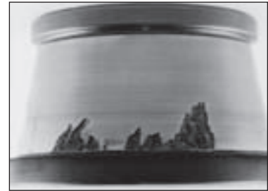
Geometric stress concentration — Spalling from misalignment, deflections or heavy loading.
