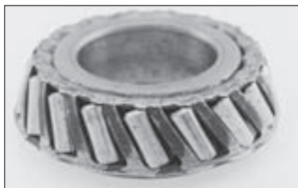
Rollers binding and skewing — Cage ring compressed during installation or interference during service.
